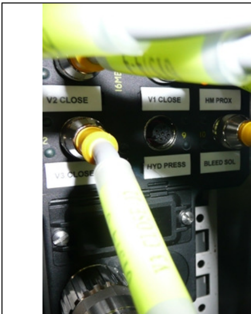
Figure 3 - Hydraulic Pressure Calibration Point
