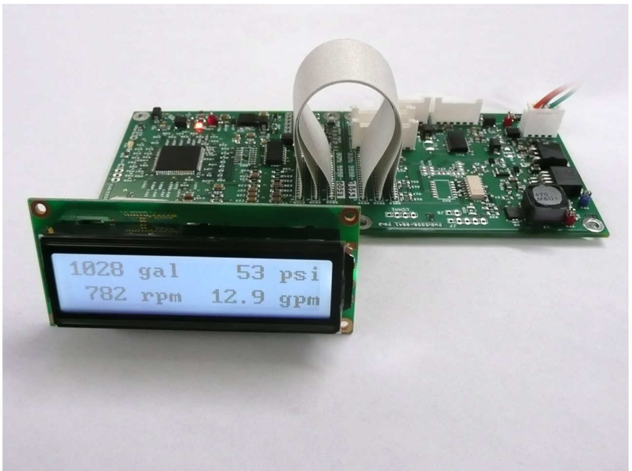
Figure 1 ~ DMS processor board, power & I/O board, and display board shown with processor board and power boards still attached.
