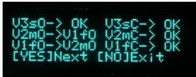
Figure 10 - Test completed and failed
