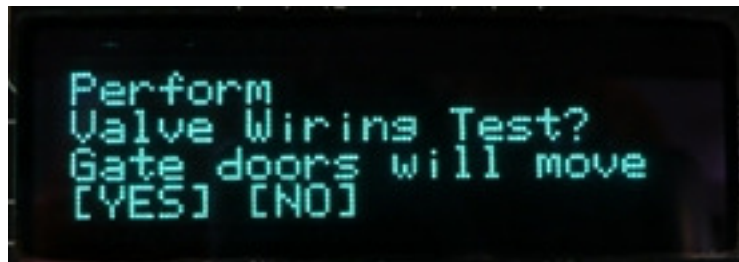
Figure 8 - Valve wiring test menu
