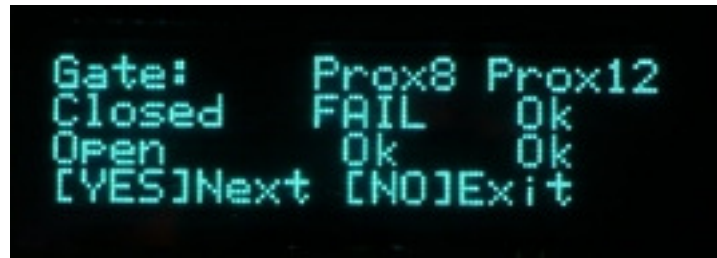
Figure 13 - Test completed and failed
